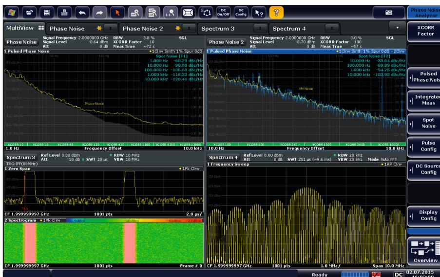
Measuring a pulsed signal in the time and frequency domain with the spectrum analyzer function.
