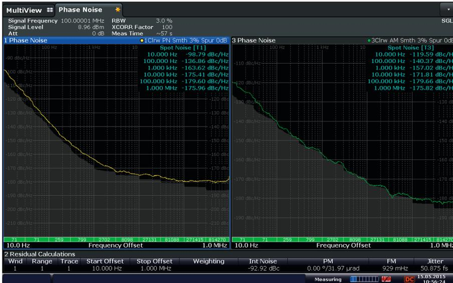
The R&S®FSWP can measure phase noise and amplitude noise simultaneously. The results can be displayed in separate windows or together in one window. (gray area: improved correlation of the R&S®FSWP, green trace: amplitude noise, yellow trace: phase noise)
