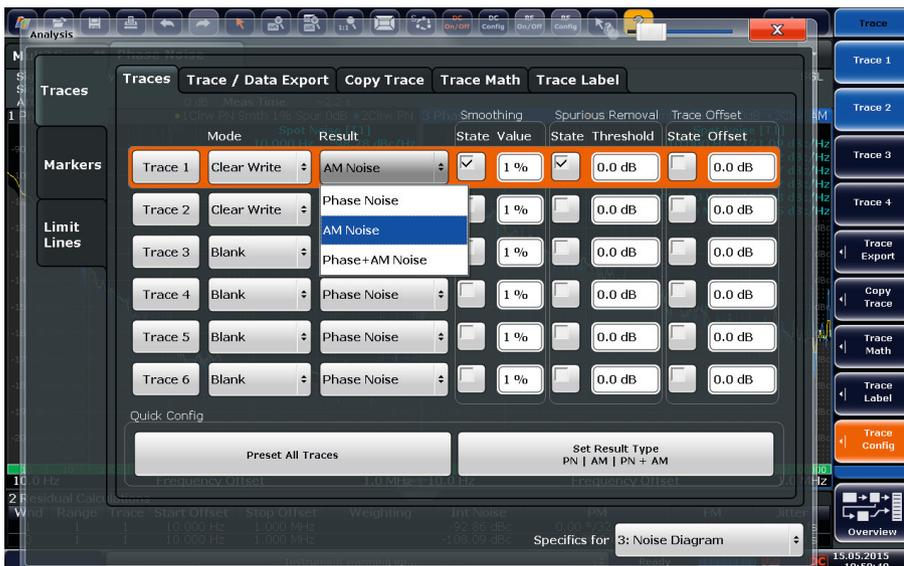
In the trace menu, users can assign traces to phase noise and/or amplitude noise measurements. They can also select whether they want spurious removed or traces smoothed.
