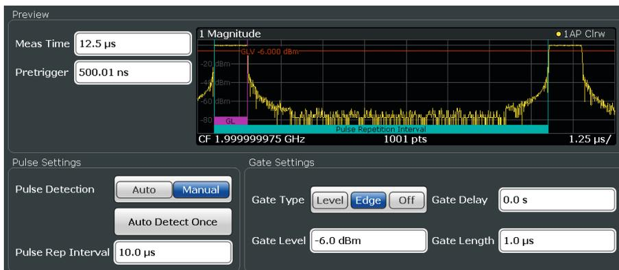
The instrument measures pulse parameters automatically; the user can define the gate.
